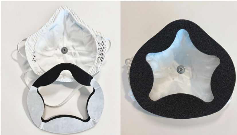
Figure 4. The ELSS-configured respirators enhanced with novel faceseal technology. The left side shows the adhesive surface with part of the backing removed. The right side shows the faceseal in place viewed from the back side of respirator.
