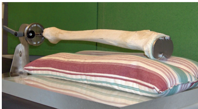
Figure 2. The human phantom bone fixed in neutral flexion on a retrograde nail in a clamp, allowing adjustment of flexion and rotation. Because the scans were made with a “spine program”, we used nylon boards and 2 long rice bags to imitate the soft tissues of the abdomen and loin.
