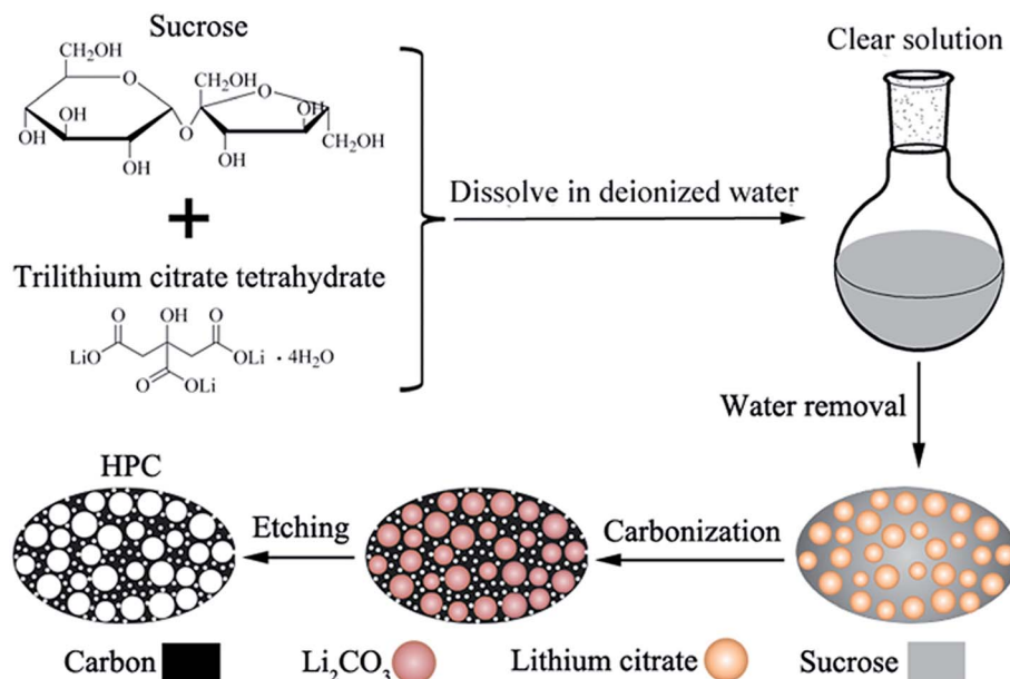
Fig. 1 Schematic drawing for the synthesis of HPC by in situ formation of template in carbon matrix.
