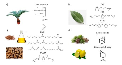
**Figure 7.** Some examples of epoxidized monomer/polymer structures derived from different biobased resources. (a) Starch-g-GMA; (b) epoxidized furanic compounds FmE, FdE, and bFdE; (c) diglycidyl furan-2,5-dicarboxylate (DGFDC) and different epoxidized fatty acid methyl esters (EMX); (d)  $\alpha$ -pinene oxide and 1,2-oxide (LMO).
