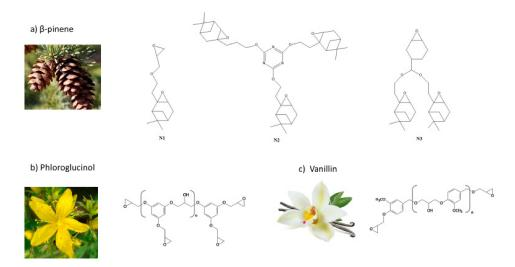
Figure 8. Epoxidized monomers derived by (a) β-pinene, (b) phloroglucinol and (c) vanillin.
