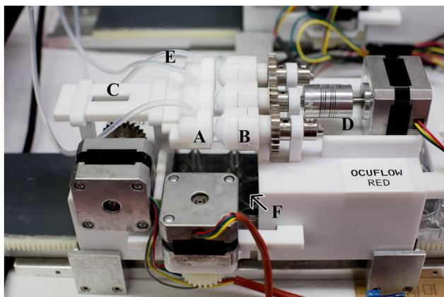
**FIGURE 1.** Features of the OcuFlow in vitro eye model: (A) corneal eye-piece and (B) lid housing the contact lens (C) lateral motion to simulate air exposure (D) rotational motion to generate frictional wear (E) Inlet for tear flow F 12-well collecting plate.
