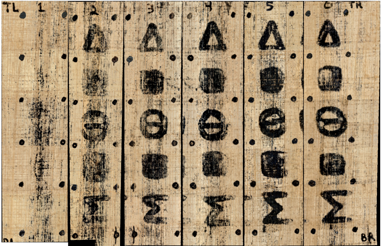
Fig 8. Photorealistic rendering of the carbon phantom scroll. This image is comprised of six training runs where one column at a time was isolated as the prediction and evaluation column.
