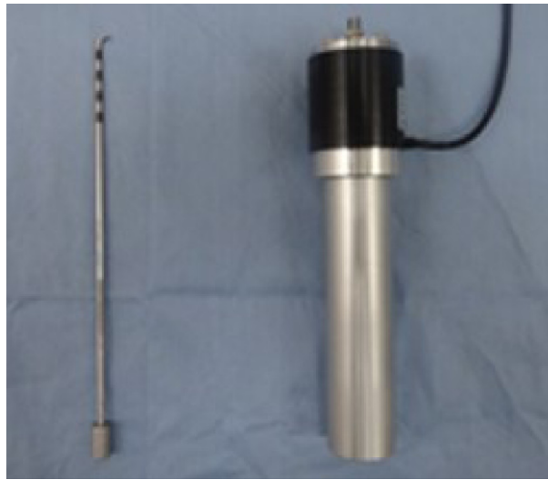
Fig. 2. Two components of the probing device in the current study. The left one is the probe with a half size. Four black marked parts in the tip of the probe to measure a distance of tissues on the monitor. The distance of each part is 5 mm. The right one is the main component to measure the force. 3-axis load cell is embedded in the black measurement part. The grip part is connected with the measurement part.
