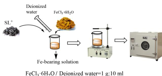
**Figure 1.** Diagram illustrating the impregnation method.
