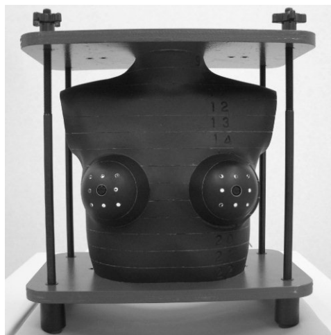
FIG. 1. The anthropomorphic female thoracic phantom used in this study. The entire phantom was cut into thin transverse sections with grids of holes for placing small dosimeters.
