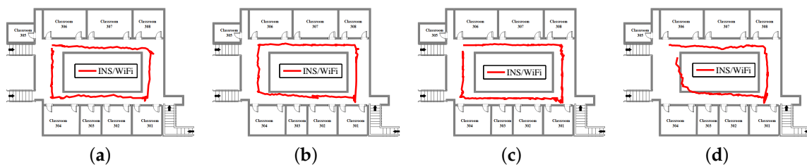
Figure 7. Positioning results for INS/WiFi: (a) calling; (b) dangling; (c) handheld; and (d) pocket.
