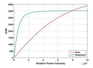
**Figure 8.** Signal-to-noise ratio (SNR) of two scan methods for light source energy dropping off in proportion.
