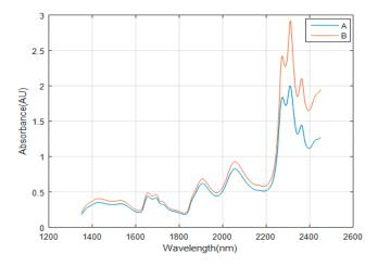
**Figure 7.** Absorbance spectrum of 95% ethanol. The blue line A is the absorbance curve of the test by the traditional scan method. The red line B is the absorbance curve of the test by the new scan method.
