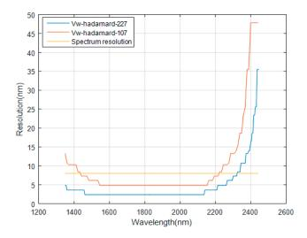
Figure 15. Digital micromirror device (DMD) resolution of the new Hadamard and the traditional Hadamard. The blue and red curves are obtained by the  $V_W$ -Hadamard mask. The yellow curve is the spectral resolution which is the same as the DMD resolution of the traditional Hadamard.
