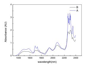
**Figure 4.** Absorbance spectrum of 95% ethanol. The blue line A is the reference spectrum tested by the UV-visible/NIR spectrophotometer UH4150. The black line B is the absorbance curve of the tested by the traditional scan method.
