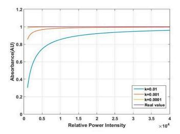
Figure 5. Influence of stray light on the low-energy wavelength band.
