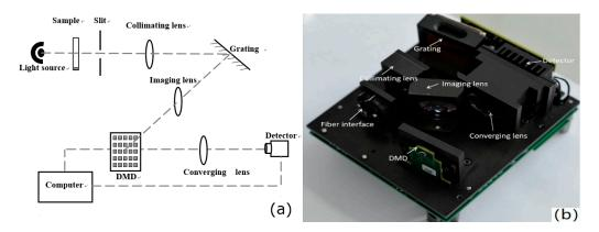
**Figure 1.** (a) Optical system of Hadamard transform (HT) spectrometer. (b) Optical structure of HT spectrometer.
