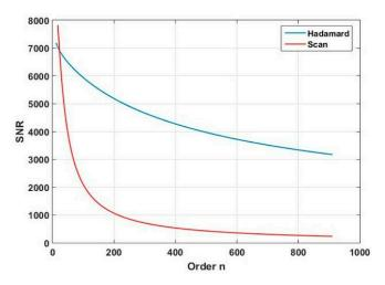
Figure 9. SNR of two scan methods for stable light source.
