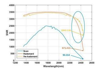
Figure 14. SNR of the spectrometer with the order of 227.
