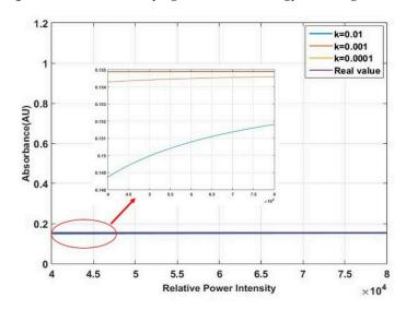
Figure 6. Influence of stray light on the high-energy wavelength Band.
