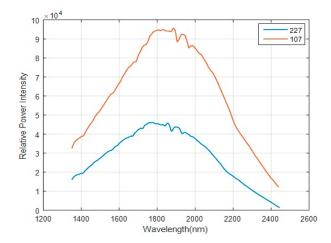
**Figure 12.** Relative power intensity of the light source. The curves are obtained by the column scan mode with the orders of 107 and 227.
