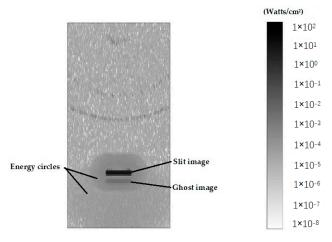
Figure 3. Incoherent radiation of slit image.
