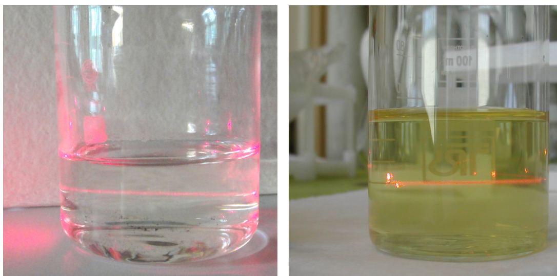
Figure 5. Light scattering (laser beam, 650 nm) by the sulfuric acid solution after a single cycle of the cellulose hydrolysis (left) and by the supernatant obtained after MCC mild mechanical treatment and centrifugation (right).
