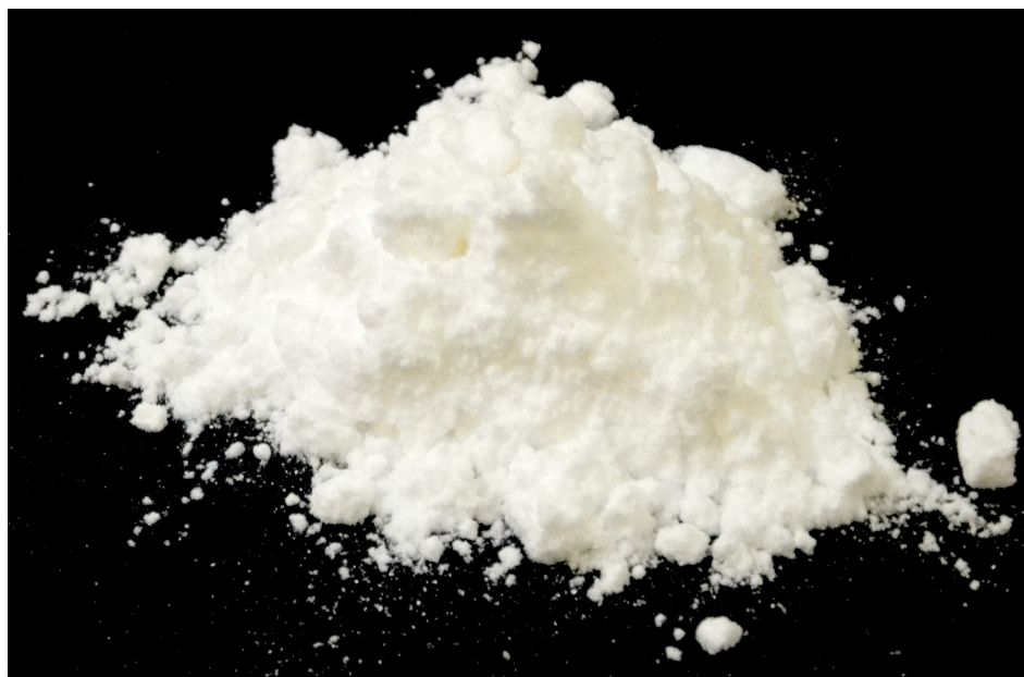
Figure 1. Microcrystalline cellulose (MCC) obtained from the hardwood cellulose raw according to the procedure described in the text.
