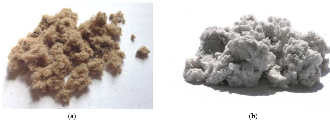
Figure 1. Appearance of finely divided technogenic fibrous materials obtained from: (a) corrugated cardboard, (b) coated writing paper.
