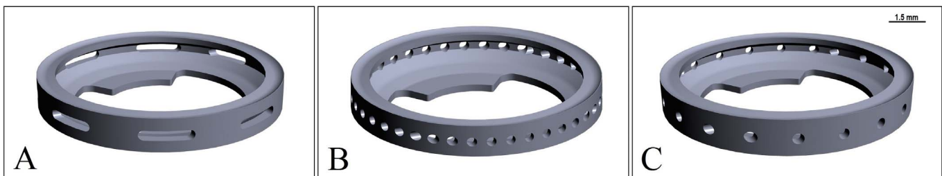
Figure 2. Schematic illustration of the different ring designs used in Part B. (A) Design RC. (B) Design RH. (C) Design RL.
