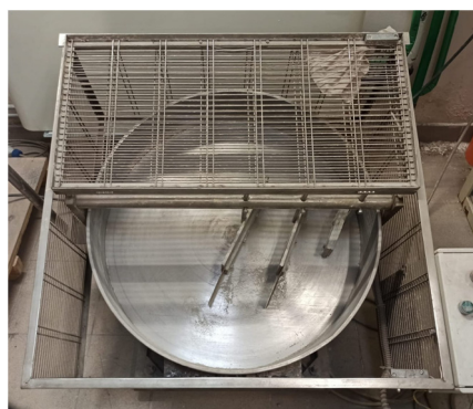
Figure 1. Cold bonding pelletization pilot-scale disk granulator.
