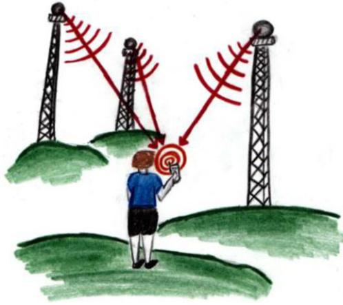
Figure 4. Finding location with cell phone triangulation. Illustration by Nichola Henne. [This figure appears in color in the online issue]
