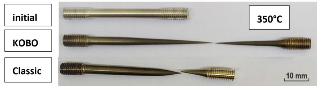
Figure 2. The appearance of samples for the tensile test and after the test.
