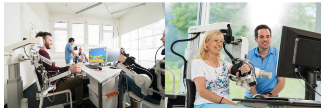
Figure 3 An example of upper limb training using an exoskeleton robot, ArmeoPower. Note: The person shown in the picture is not a patient and was taken with the participant's knowledge and permission. Picture courtesy: Hocoma.
