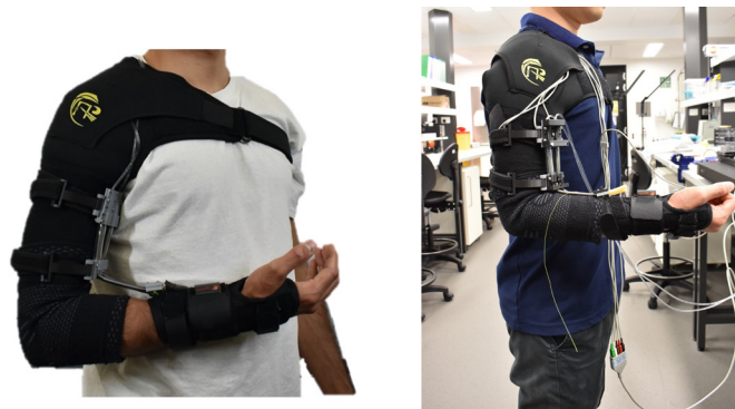
Figure 4 An example of an upper limb exosuit robot described by Hoang et al 7 being worn by a volunteer. Note: The person shown in the picture is not a patient and was taken with the participant's knowledge and permission. Picture courtesy: Dr Thanh Nho Do.
