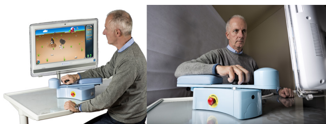
Figure 2 An example of upper limb training using an end effector robot, MO.TO.RE. Note: The person shown in the picture is not a patient and was taken with the participant's knowledge and permission. Picture courtesy: Humanware S.r.l.
