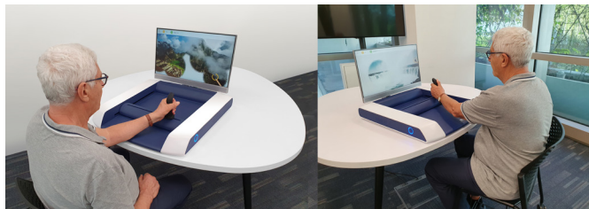
Figure 1 An example of upper limb training using an end effector robot, H-man. Note: The person shown in the picture is not a patient and was taken with the participant's knowledge and permission. Picture courtesy: Articares.
