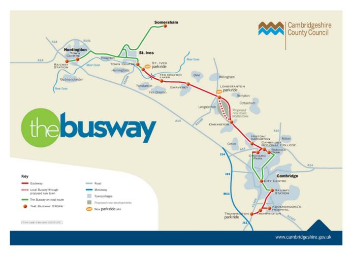
**Figure 1. The Cambridgeshire Guided Busway.** Reproduced with permission from Cambridgeshire County Council and Stagecoach. The guideway runs from St Ives to the northern edge of Cambridge city, and from Cambridge railway station south to Addenbrooke's Hospital and Trumpington. Through the city centre, and north of St Ives, guided buses join the road network. doi:10.1371/journal.pone.0069254.g001
