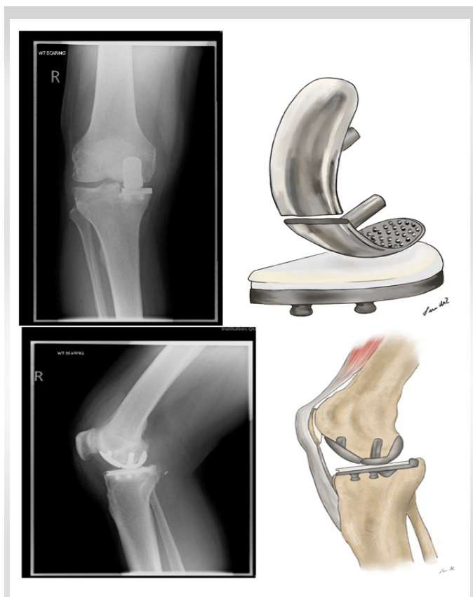
Figure 1: Two-dimensional X-ray and illustration of the right knee showed unicompartmental knee arthroplasty fractured of the femoral component.
