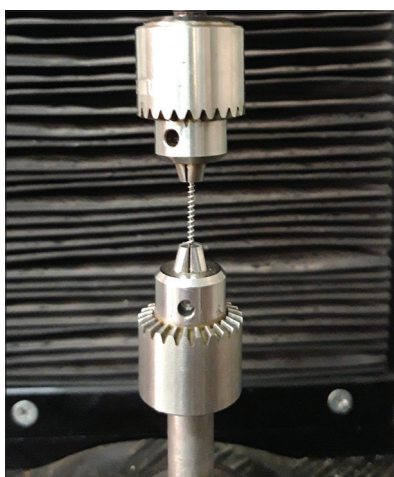
Figure 1: Measuring unloading force of each coil.
