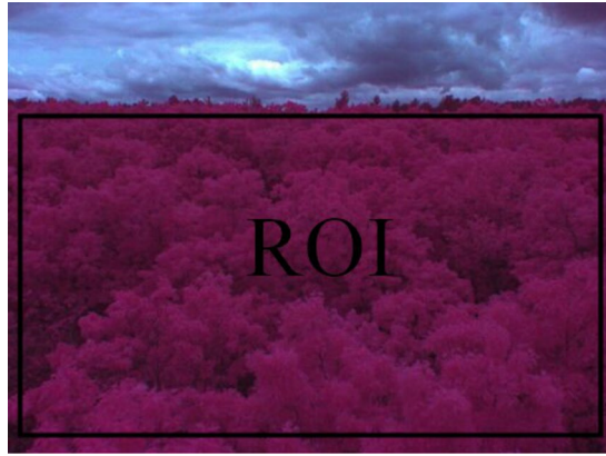
Figure 6. The example of an infrared image on September 19 th , 2014. The black rectangles indicate the Region of Interest (ROI) used to calculate camera-NDVI. The ROI includes approximately 2,800,000 pixels. Because plants absorb much red light and reflect a lot of infrared light, this NDVI camera makes near infrared wavelengths visible as red while red wavelengths appear as green and green as blue, and thus produced a new color-infrared (CIR) image. On CIR imagery vegetation appears red.
