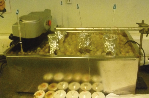
FIGURE 1: Experimental set-up for isothermal leaching of potato samples.
