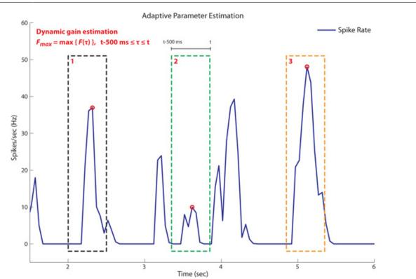
**Figure 6:** Adaptive controller gain. The proportional controller uses a static gain, Kp, whereas the adaptive controller estimates the gain continuously during closed loop control. The dynamic gain, Kp, is inversely proportional to the maximum spike rate, Fmax, over the interval t-500ms  $\leq \tau \leq t$ . Figure shows three instances where Fmax is estimated over time. Based on estimated values of Fmax, Kp is highest during time window 2 (green) and lowest during time window 3 (orange).
