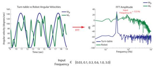
**Figure 4: Frequency response.** Angular velocity signals for the turn-table, ωp, and robot, ωr, are transformed into the frequency domain using the fast Fourier transform (FFT) method to calculate amplitude and phase components at the input frequency. Phase components of FFT are not shown in the figure.
