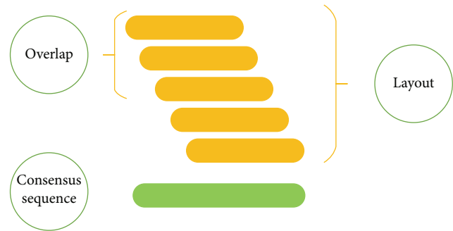
FIGURE 2: De novo assembly: reads that overlap each other are shown to align at appropriate places with respect to one another, thereby generating the layout . The layout, in turn, constructs a consensus sequence, simply by basing itself on the majority base call. The above-mentioned framework is called “ Overlap-Layout-Consensus .”
