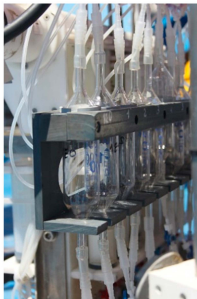
Figure A3. The set of gas-impermeable glass ampoules for water sampling for the analysis of dissolved gases.
