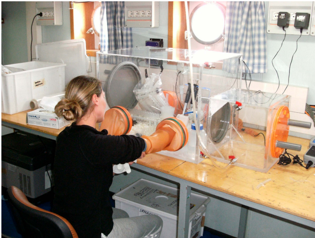
Figure A4. Filtering, subdivision into aliquots, and treatment of the water samples collected by the syringes of the Amerigo Lander is conducted in a Nitrogen glove-box.
