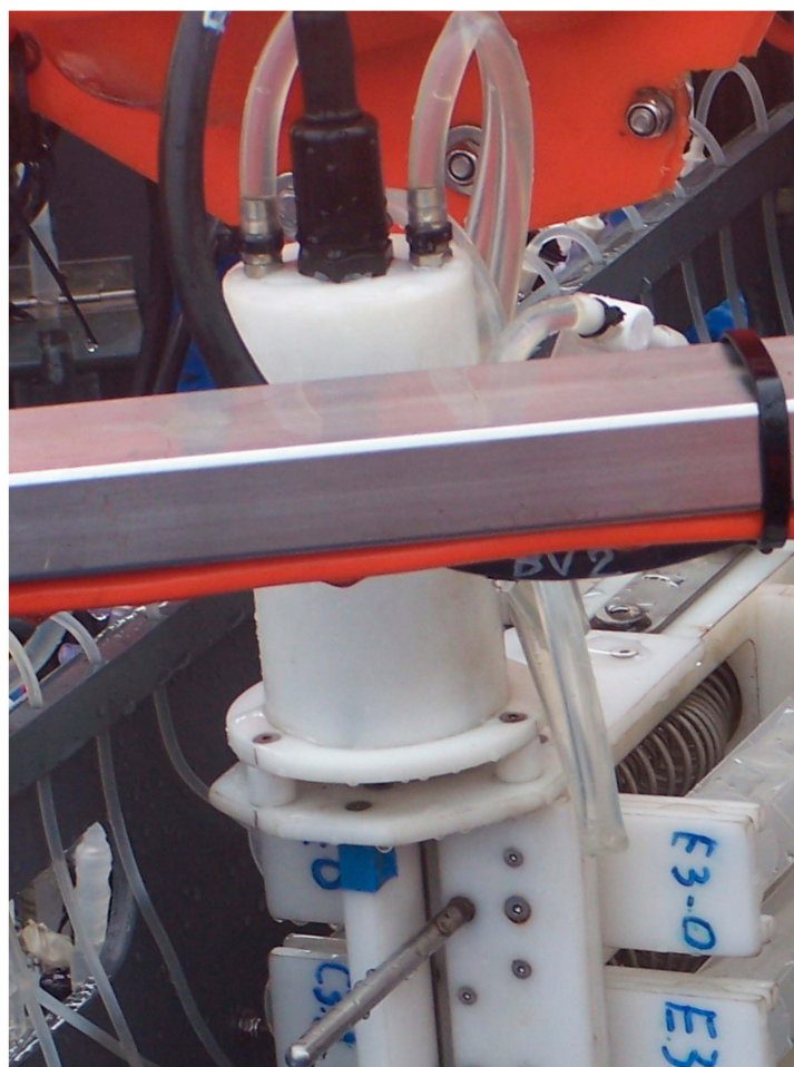
Figure 12. The Delrin case hosting the electric motors with the silicone tube pressure-compensation system.
