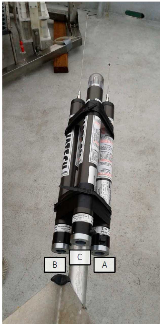
Figure 6. Amerigo Lander recovery system. (A) GPS localization (Novatech ARGOS Beacons); (B) directional radio localization system (Novatech Radio Beacon); and (C) flash for visual localization at night (Novatech Xenon Flasher).
