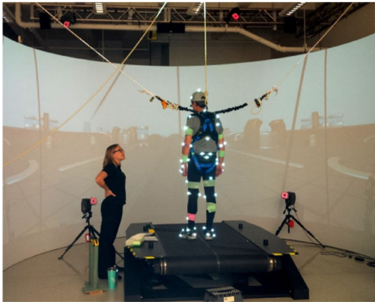
Figure 1. An example image of the research study performed in the laboratory. The participant is standing on a dual-belt treadmill and wearing 54 reflective markers that are being captured by 12 surrounding cameras.
