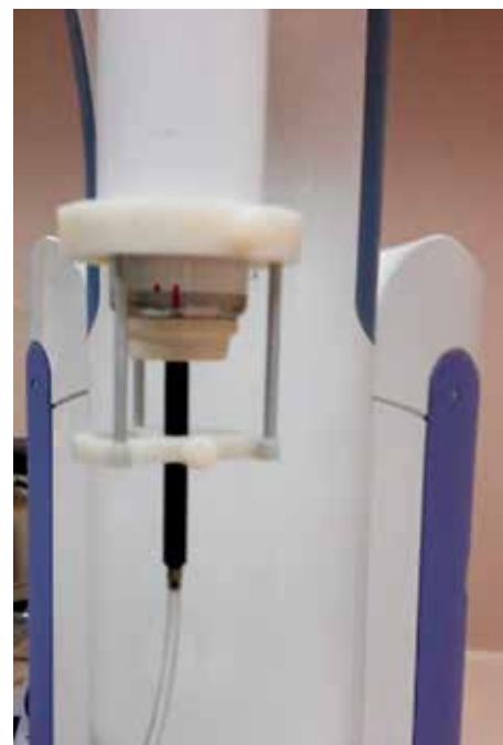
Fig. 1. Setup for measurements with the Exradin A20 ionization chamber
