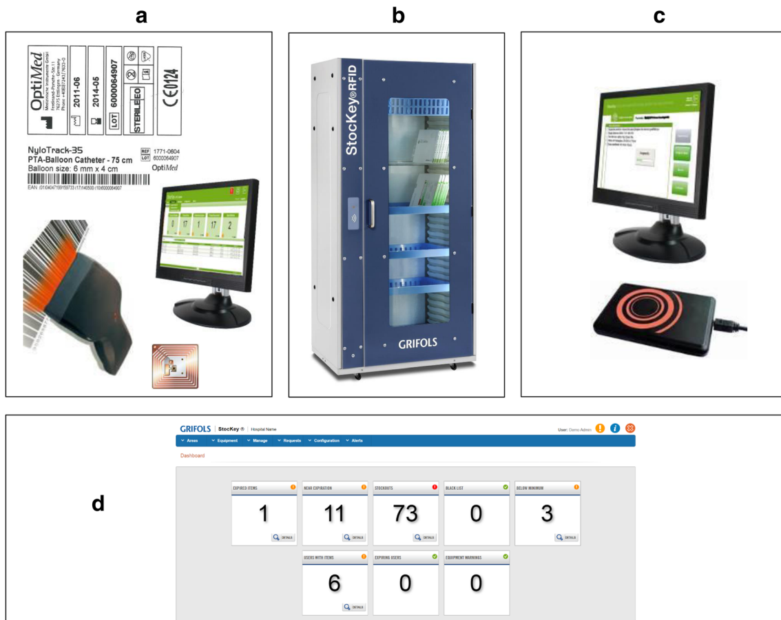
Fig. 1 The RFID Smart Cabinet components: A) labeling station; B) Closed cabinet; C) Patient assignment station; D) Dashboard with KPI's (Key Performance Indicators) and integrations with the Hospital Informatics System
