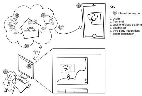
**Fig 1. Major components of a web application (web app).** In this line drawing, the (a) user is shown interacting with the (b) front end of the web app. The front end is updated based on changes that occur in the back end (c and d). Updates that occur in the back end can also trigger other actions, such as (f) text or email notifications via (e) third-party integrations. *Image credit: Sheila M. Saia (CC BY 4.0).*
