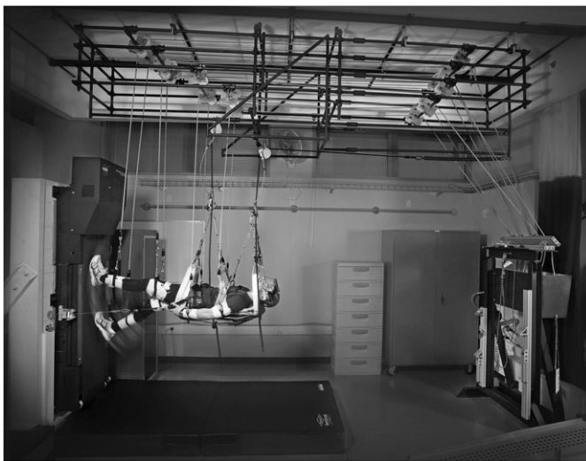
Fig. 1. The zero-gravity locomotion simulator (ZLS) in which subjects assigned to the exercise group walked and ran during the study. Subjects assigned to the control group were suspended in the ZLS for a similar period of time but did not exercise.
