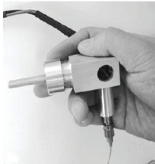
FIGURE 2: Arthroscopic OCT probe. (a) A schematic diagram of the OCT probe. (b) A photograph of the hand-held OCT arthroscopy probe. PBS, polarization beam splitter; CM, fiber optic collimator.
