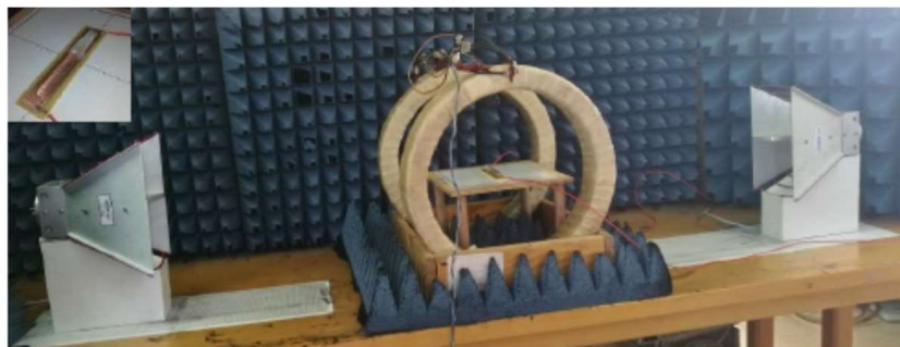
Figure 2. Experimental set-up for frequency and time domain measurements including emitting and receiving antennas, Helmholtz coils and detail of magnetic microwire inside of a capillary on a heating resistance. Insert: Detail of magnetic microwire inside of a capillary on a heating resistance.
