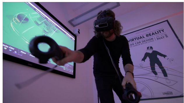
Fig. 6 A car is being designed on a 1-to-1 scale with RealityWorks (courtesy of SeymourPowell)
