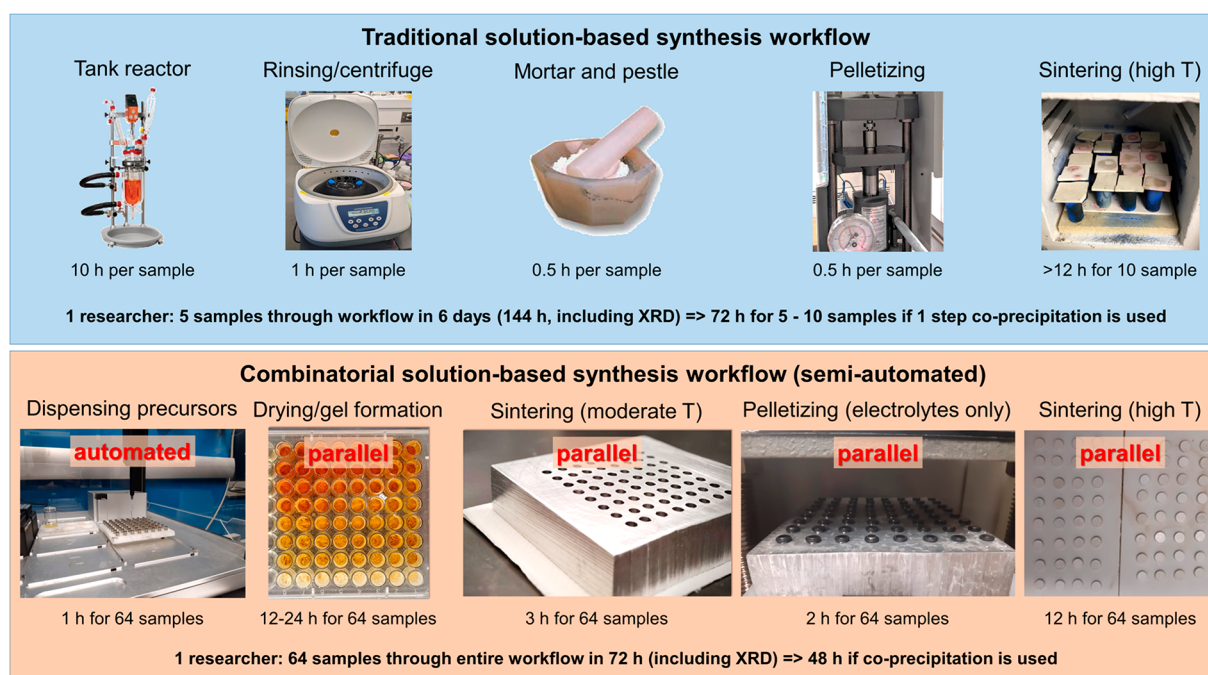
Figure 4. Comparison of traditional solution-based synthesis workflows to the semiautomated method used in the McCalla lab. Time estimates for the traditional workflow are based on the author's experience in various battery research laboratories where coprecipitation is performed in a tank reactor. The 1-step coprecipitation approach involves performing the coprecipitation rapidly in a beaker as described in ref 39. Portions reproduced from ref 46. Copyright 2022, Canadian Science Publishing.
