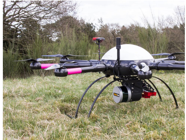
FIGURE 1 UAS LiDAR system with background of Cytisus scoparius shrubs. Photo credit: Urs A. Treier
