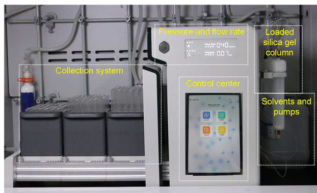
Figure 4. Rapid separation and purification instrument: AutoSepa-MJL
