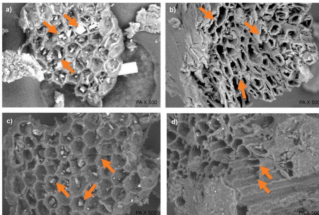
**Fig. 8.** SEM micrographics. a) Control bagasse, b) bagasse with acid pre-treatment (A10-1.5), c) bagasse with enzymatic pre-treatment (E24-1.5), d) bagasse with acid-enzymatic pre-treatment (E6-1.5).
