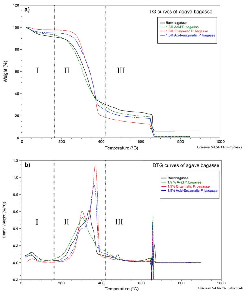
**Fig. 9.** a) Thermogravimetric curves of agave bagasse. b) thermal decomposition characteristics curves of ATW. Raw bagasse (black), with a 1.5% acid pre-treatment for 10 min (green), with a 1.5% enzymatic pre-treatment for 6 h (red), and with a 1.5% acid and enzymatic pre-treatment (blue). (For interpretation of the references to colour in this figure legend, the reader is referred to the Web version of this article.)
