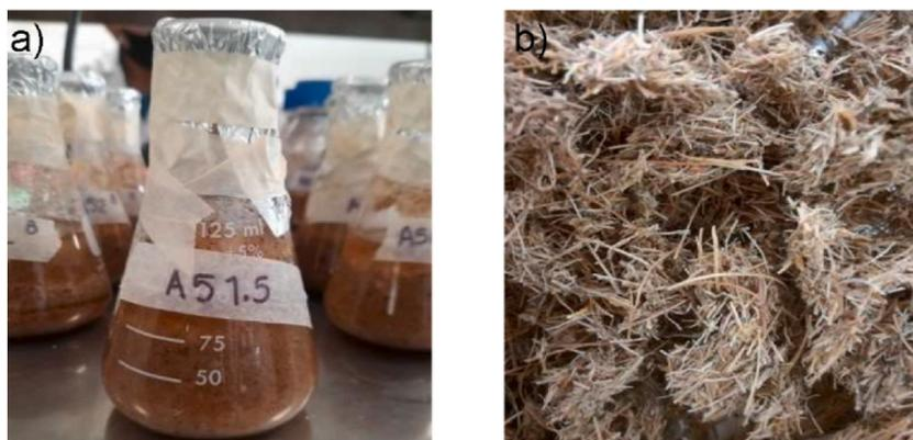
Fig. 2. a) Acid pre-treatment of agave bagasse. b) Agave bagasse after acid pre-treatment.
