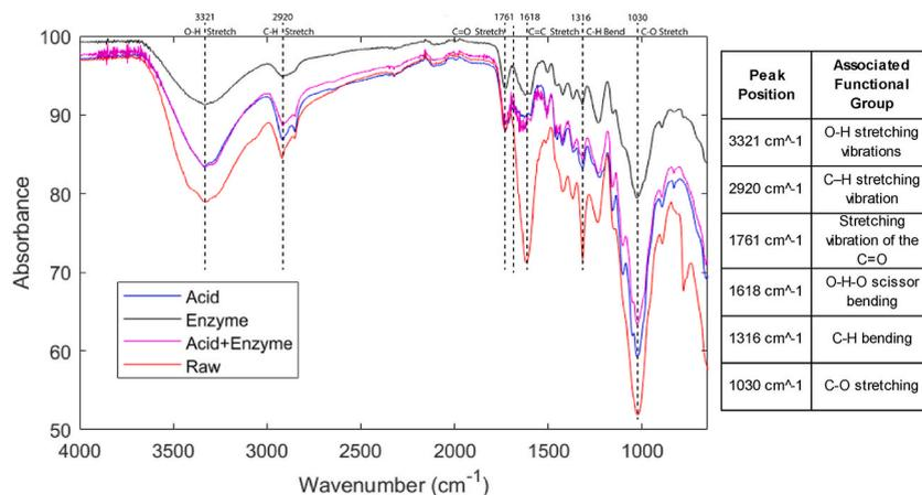
**Fig. 7.** FTIR spectra of ATW untreated (red), 1.5% concentration acid pre-treatment for 10 min (blue), 1.5% concentration enzymatic pre-treatment for 6 h (black), and acid-enzymatic pre-treatment (1.5% acid concentration for 10 min, 1.5% enzymatic pre-treatment for 6 h) (pink). Peaks are shown in the table to the right. (For interpretation of the references to colour in this figure legend, the reader is referred to the Web version of this article.)
