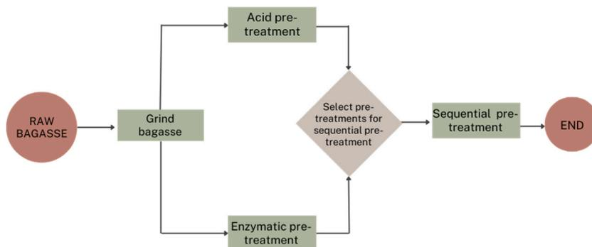
Fig. 1. Pre-treatment process diagram.
