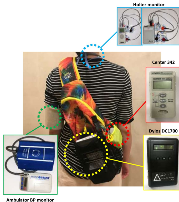
Figure 1. Study devices for the study. A study subject carries four study devices for 24 h: Dylos DC1700 for PM_{2.5} monitor, Center 342 to monitor the temperature and humidity, Holter monitor, and an ambulatory blood pressure monitor.
