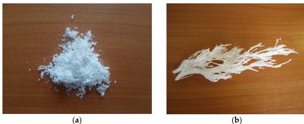
Figure 3. SAS formation of polycarbonate (PC) powder at 1 mL/min (a) and PC icicles at 2 mL/min (b).
