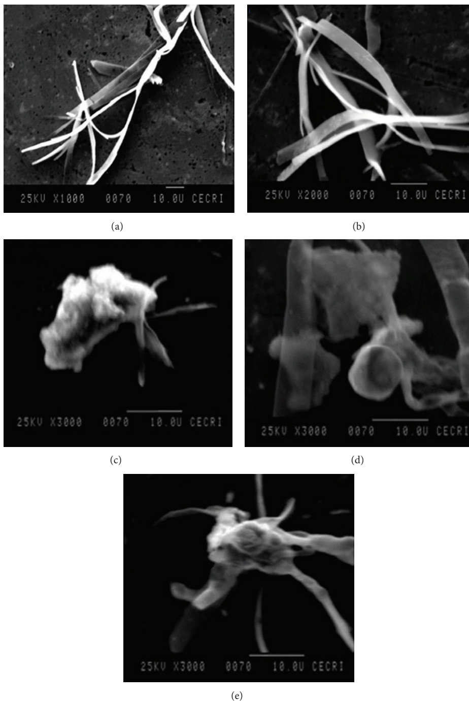
FIGURE 7: SEM images of (a) and (b) BEF ligand, (c) BEF-Cu, (d) BEF-Ni, and (e) BEF-Zn.
