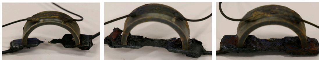
Figure 14. The three corrosion sensors after accelerated corrosion failure.
