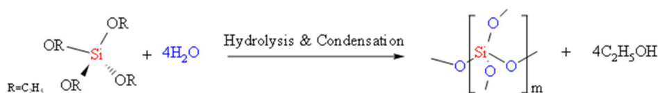
(b) Crosslinking reaction of Hy-PDMS and TEOS
