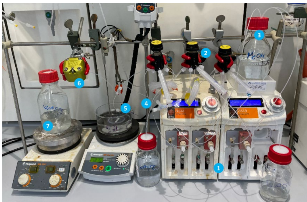
Figure S3. Photograph of the flow setup. Legend: (1) Syringe pumps (P1, P2 and P3), (2) reagent feeds with injection valves and two sample loops, (3) carrier solvent, (4) Y-mixers, (5) reaction coil in a heated oil bath, (6) adjustable BPR, (7) reactor outlet.
