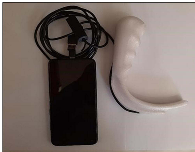
Figure 2 The novel device used in this study. The 3D printed VL blade and handle are attached to a commercially available 6.5 mm borescope camera inserted into a Samsung ® Galaxy A11 smartphone.
