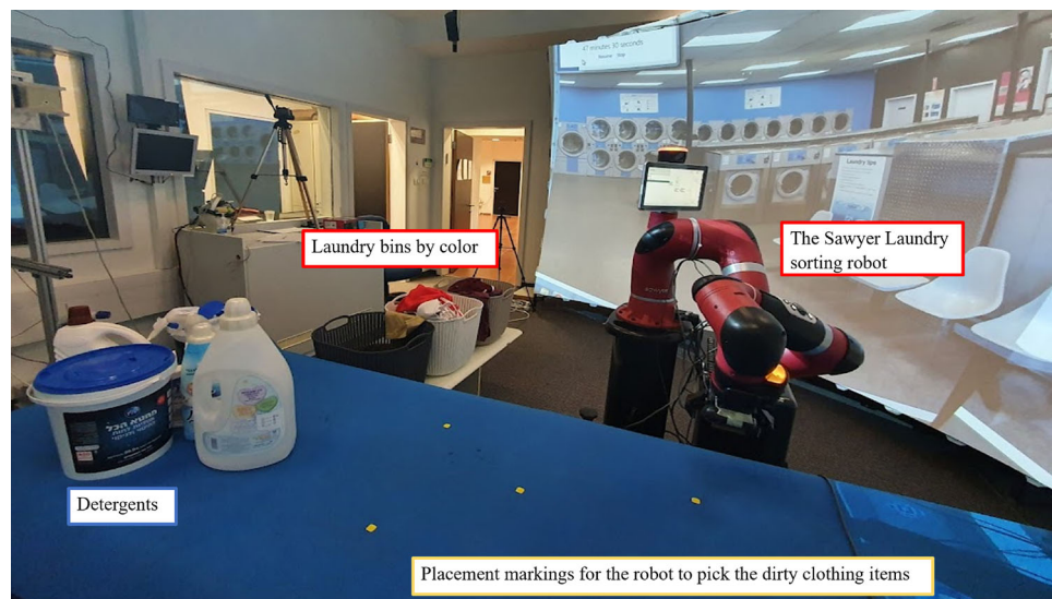
Fig. 1 The laundry sorting workstation of the robot from the perspective of the participant. Participants stood on the opposite side of the laundry sorting table. To their right was a table with a pile of clothes (not seen in the image)
