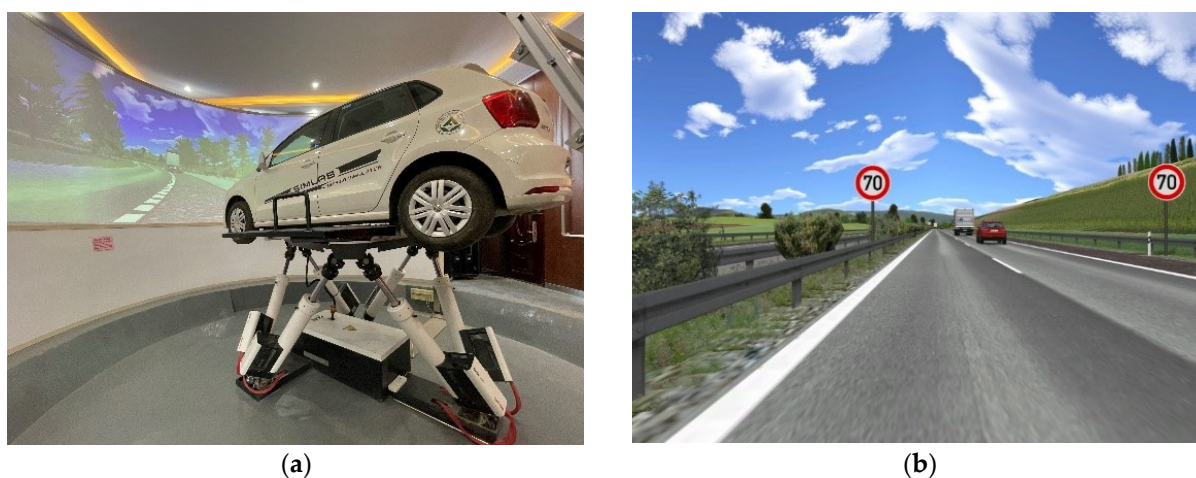
Figure 1. Driving simulator: (a) 6-DOF driving simulator; (b) the scenario of driving simulating software.
