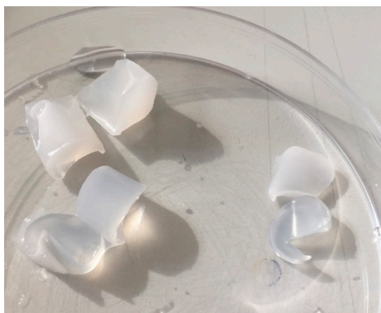
Figure 7. Picture of the potato starch hydrogels obtained in this investigation at fixed conditions (starch-water concentration of 20% w/w, mean size of <25\ \mu\text{m} and processed at 600 MPa for 15 min at 50\ ^\circ\text{C} ).
