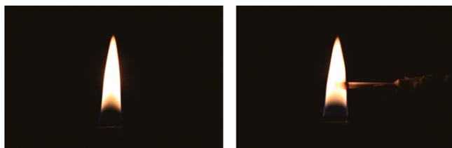
Figure 14. Original flame shape and the flame shape when the probe is inserted into it by using probe sampling.
