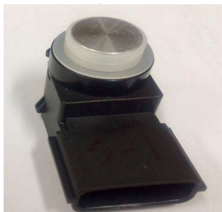
Figure 11. An actual ultrasonic sensor for in-air applications.
